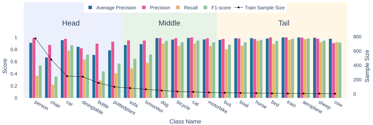
FIGURE 6. Average Precision, Precision, Recall, and F1-score per class of LM-CLIP on VOC-MLT. The used vision encoder is ViT-B/16. We use a threshold of 0.5 after a softmax on the prediction scores to calculate precision/recall. This graph is omitted for COCO-MLT, as it cannot be reasonably plotted for 80 classes.
